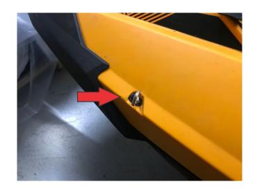
Photo: example, BRP Spark bolts position **F** – FRONT
