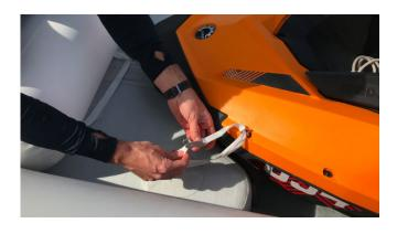
Inflate front tube-fence and secure it with the webbing on the bottom or on the side according to the preparations on the main hull.
